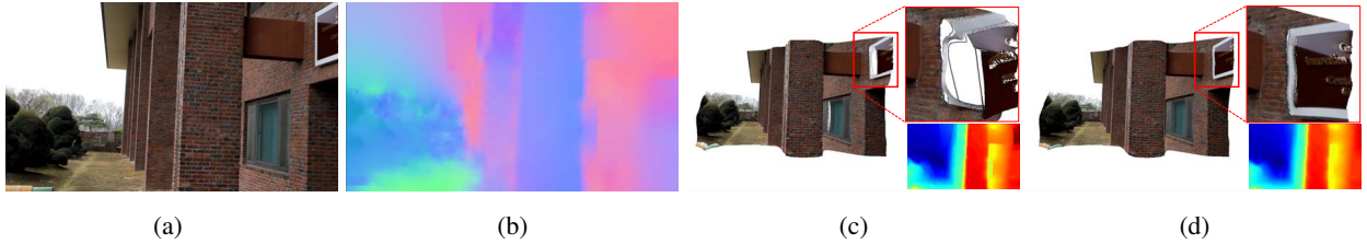
Figure 6. Dense reconstruction result with/without geometric guidance - Building2 . (a) Reference image. (b) Estimated normal map. (c) 3D mesh and depth without geometric guidance. (d) 3D mesh and depth map with geometric guidance.
